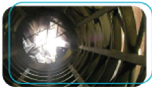
RCR trommel Screen Nukote ST-M 6mm internal
